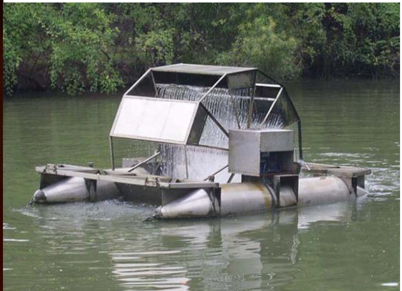
Chaipattana Low Speed Surface Aerator for waste water treatment
