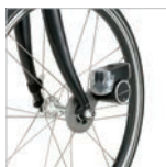
A generator device is attached to produce electricity
