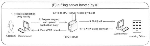
ePCT-Filing transmits the application to a server hosted at the International Bureau on behalf of the receiving Office. The receiving Office is notified when a new international application was filed and manages the international applications through a web interface similar to that provided for applicants. Although the International Bureau technically maintains the server, the receiving Office remains responsible for processing the international application.
