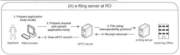
ePCT-Filing is fully compatible with existing e-filing servers according to the current e-filing standard. ePCT-Filing transmits the application to the receiving Office in exactly the same format and using the same transmission protocol as PCT-SAFE. Receiving Offices already operating such a server will not need to make any changes to their IT systems or procedures. They can continue to accept filings from PCT-SAFE or other compatible software in addition to ePCT-Filing.
