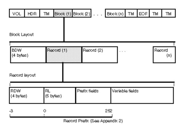
VOL = Tape volume id HDR = Header records EOF = End of file records
